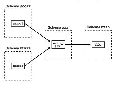
Figure 8–2 Indirect Calls to an Invoker's Rights Subprogram
