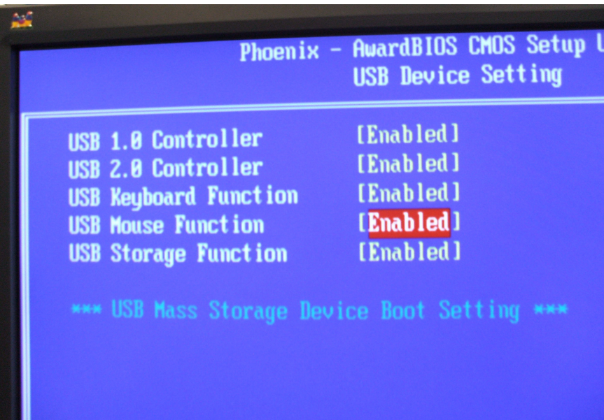
Figure 10-15 USB Device Setting screen
