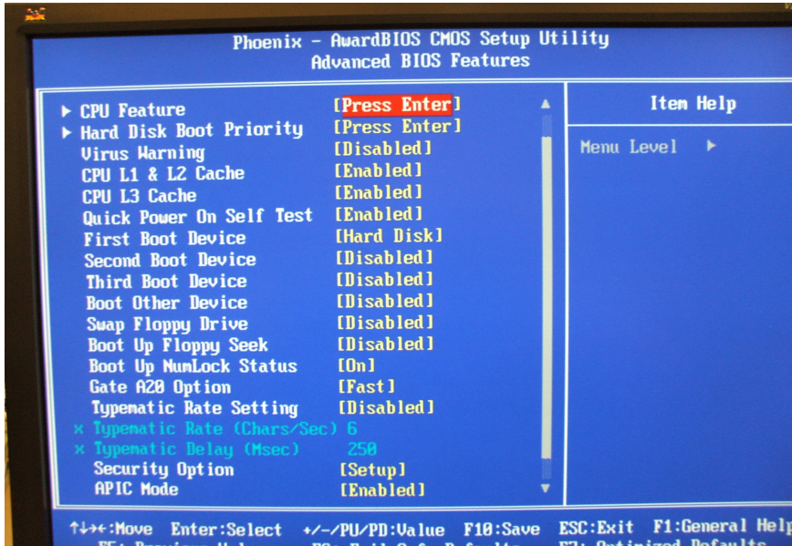
Figure 10-7 Advanced BIOS Features screen (Part 1)
