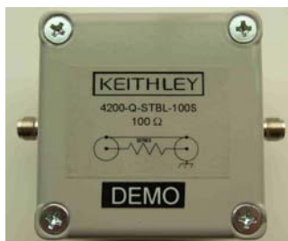
Figure 11. Photo of one of the stabilization resistors, showing the SMA connections on either side.
