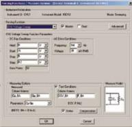
The Model 4200-CVU is an integrated instrument designed to plug directly into the 4200-SCS chassis, so it can be controlled through KITE's point-and-click interface, just like an SMU, and allow users of any level of experience to perform C-V testing as if they were experts. A variety of sample tests, including tests for MOSCAPS, MOSFEIS, and Mobile Ion characterization are bundled in, as well as common
