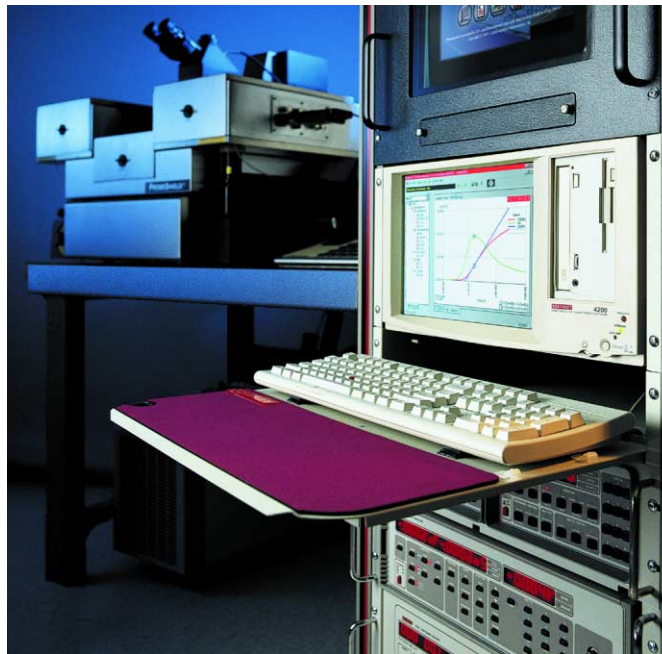
Figure 4. Example of a Windows®-based semiconductor characterization system, the Keithley Model 4200-SCS.
